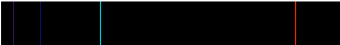
Figure 4: Hydrogen emission spectrum. Note only certain wavelengths are produced
